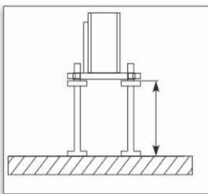
3. Put this assembly on the floor and prepare a rough surface for proper bonding of grouting.
