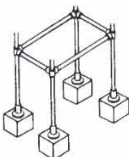
⑦ Grout the foundation bolts and fix the structure bases with that.
