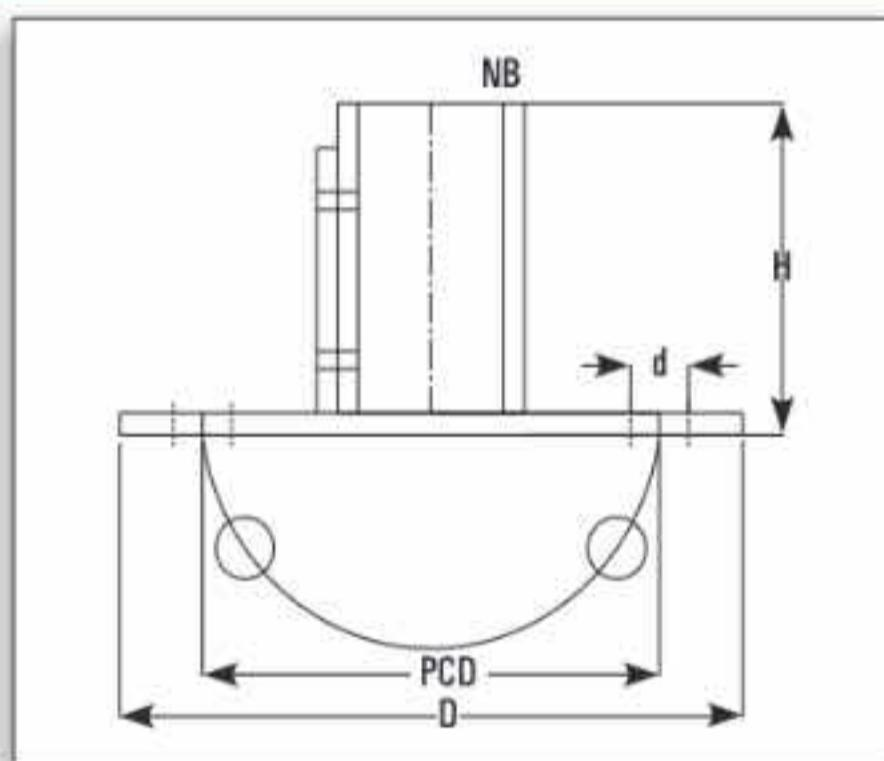
These are to be used with vertical tubes. Holes are provided for foundation.
