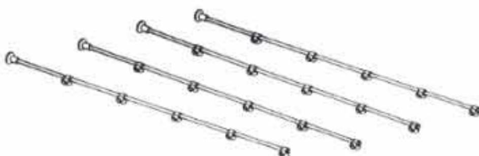
① Mark the position of required fittings on all the Vertical tubes, slide them in correct sequence and lightly Tighten.
