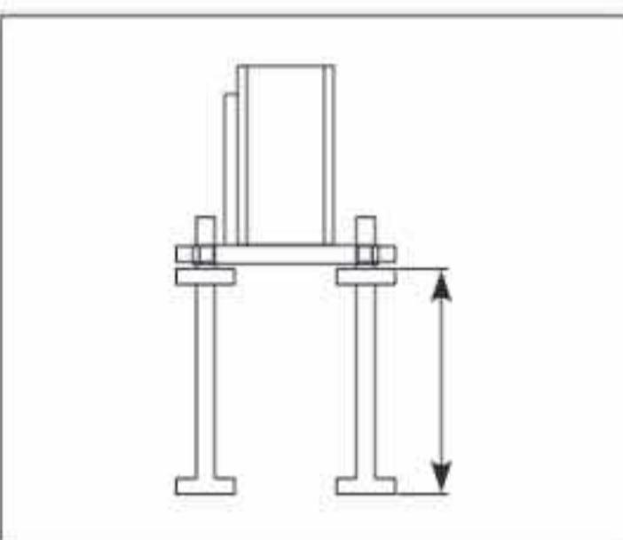
2. Fit the bolts in BASE so that base is raised upto 150mm from head of bolts.
