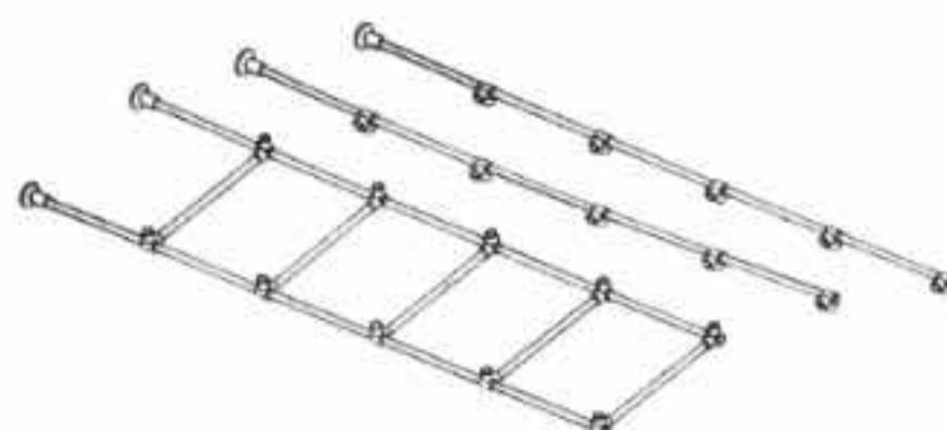
② Assemble one side frame of the structure by adding the cross tubes between two vertical tubes.
