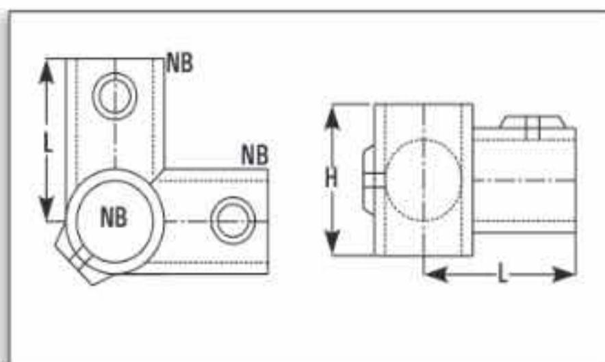
These are used to build frames on vertical tubes.
