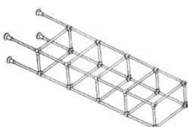
⑤ Add the other side frame on it and tighten all the fittings firmly.
