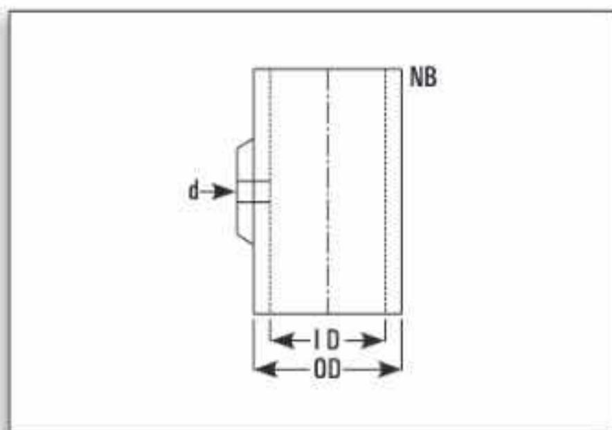
Following structure fittings are available to use with galvanised tubes in order to form a tubular structure for a glass plant. These fittings are made of cast iron. Also available in Stainless Steel 304 & 316 and are suitable to the galvanised tubes described earlier.
