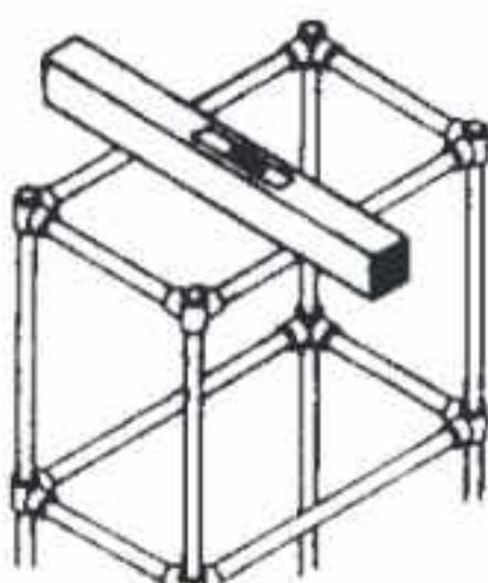
⑨ Adjust the horizontal frames in correct level.
