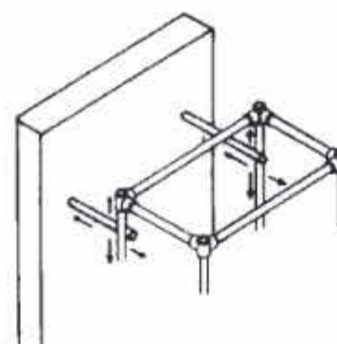
⑧ Adjust bracing to obtain a correct plumb in Structure.
