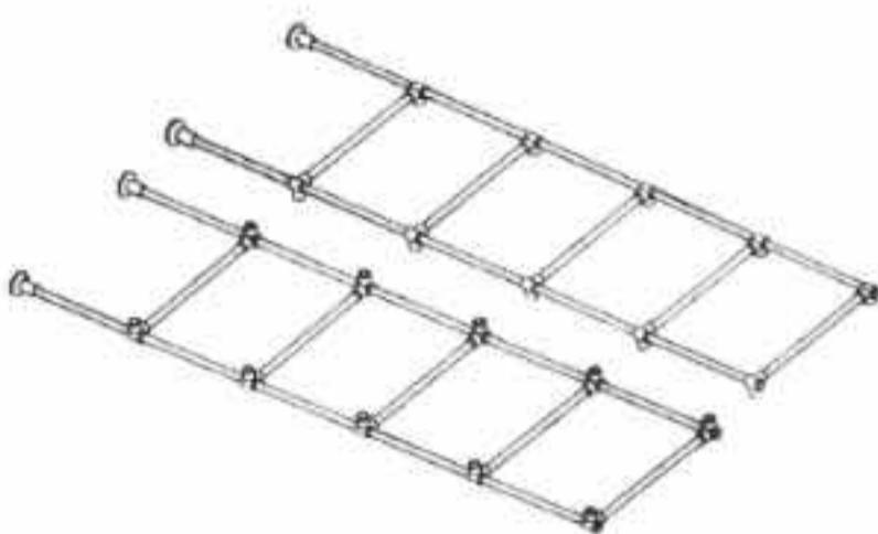
③ Assemble other side frame of the structure by adding the cross tubes between other two vertical tubes.
