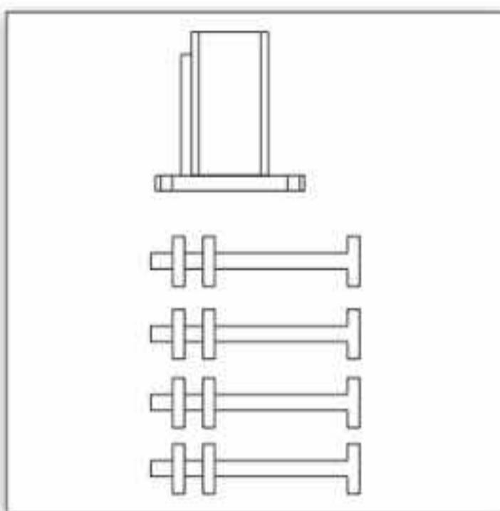
1. Take one Cast Iron BASE and four foundation Bolts, each with 2 nuts.
