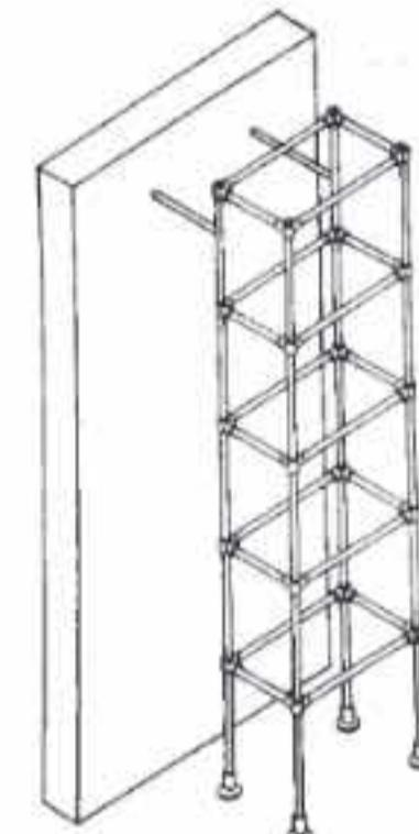
⑥ Hoist the structure and brace it to some existing rigid feature.
