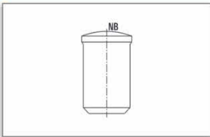
These are used to plug the open ends of galvanised tubes.
