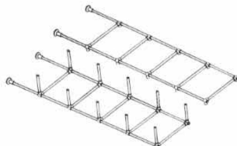
④ Build up the cross tubes in one side frame and Tighten lightly.
