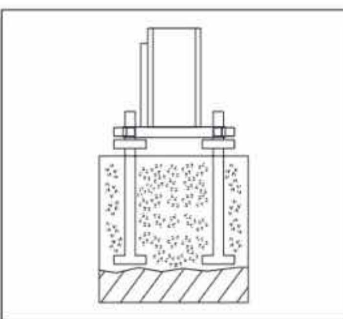
4. Make a concrete block over the bolts of about 200 x 200 mm upto the base of BASE i.e. 150mm high.
