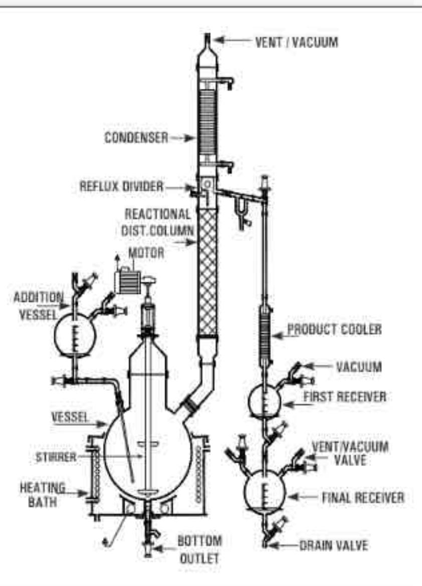
This is a versatile unit and can be used as Reaction Distillation Unit, Fractional Distillation Unit or a combination of both. All features of Reaction Distillation Unit and Fractional Distillation Unit are incorporated.
