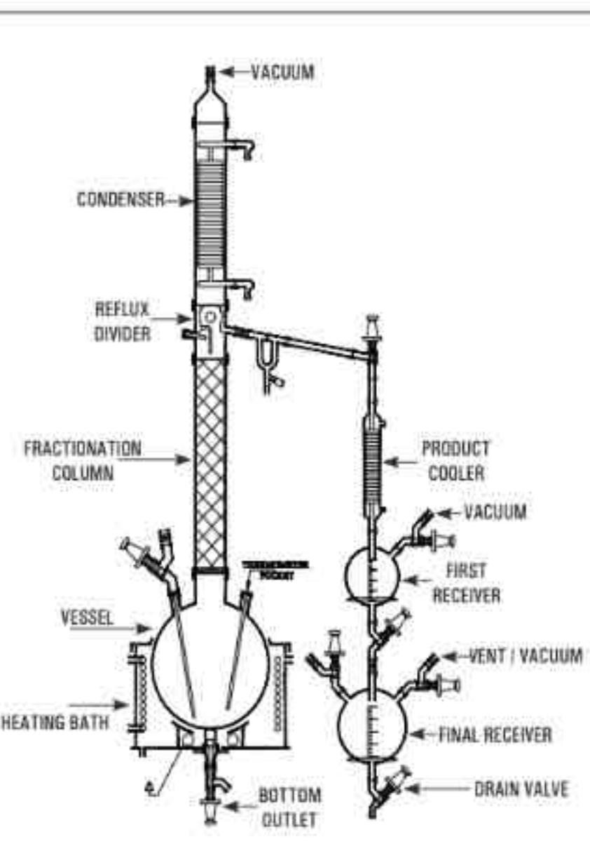
This is essentially a compact batch-type fractional distillation unit in which the reboiler consists of a vessel mounted in a heating bath and with a packed column above. The vapours from top is condensed and can be refluxed as per requirement.
