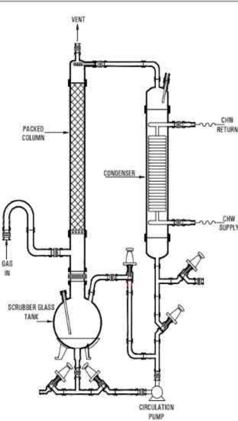
Goel offer Pilot Plant Gas Scrubber for various gases like HCl, Cl<sub>2</sub>, SO<sub>2</sub>, Br<sub>2</sub>, HBr, NO<sub>x</sub> etc or any other corrosive gases. These scrubbers use the media as water / Aq. NaOH / any other suitable solvent which can neutralise the exhaust gases. Our Pilot plant scrubber are ranging from 20L vessel capacity to 500L vessel capacity and scrubber diameter from 80DN to 300DN.
