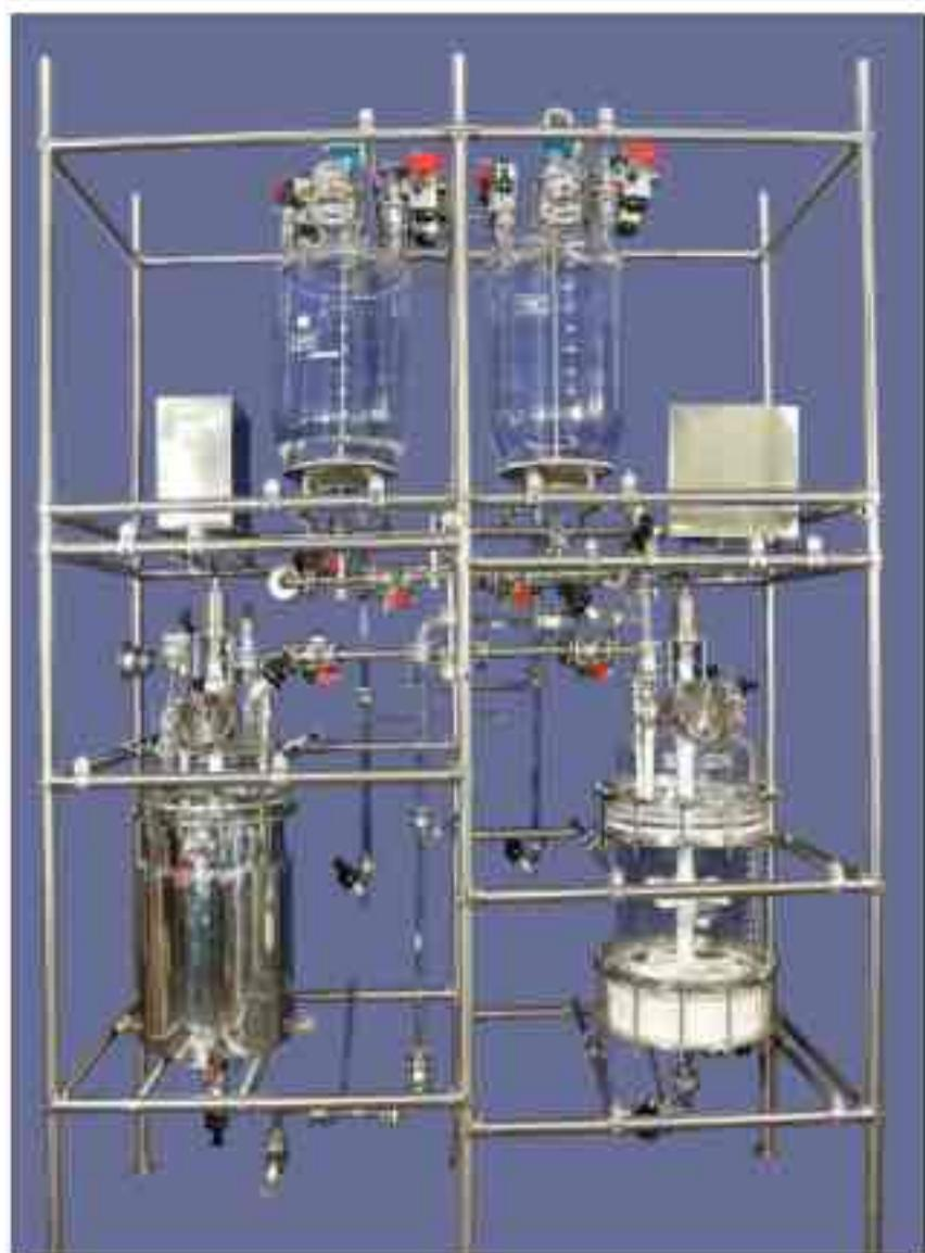
Agitated Glass Nutsche Filter is a closed vessel designed to separate solid and liquid by filtration under vacuum. The closed system ensures odourless contamination free and non-polluting working conditions maintaining product purity and hygiene. Agitated Nutsche Filters are extensively used in Herbal products, Chemical product development, kilo lab operation, pharmaceutical manufacturing, agro chemical and the food industry.
